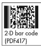
Two-dimensional bar codes (2-D)—such as PDF417, Maxicode, and DataMatrix—are scanned horizontally and vertically. They hold considerably more data than 1-D bar codes. The 2-D bar code can expand the number of characters from approximately 20–30 in 1-D bar codes to more than 2,000.1 A 2-D bar code can thus contain the contents of an entire document.
